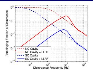
Ability to reject disturbance depends its on frequency! Frequencies around 100 kHz are worst!
