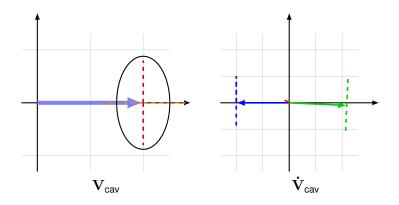
Small beam loading, disturbance due to modulator ripple only affects cavity phase  $\Rightarrow$  amplitude and phase requirements are OK
