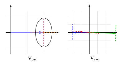
Disturbance due to modulator ripple affects mostly cavity amplitude, disturbance due to modulator ripple only affects cavity phase  $\Rightarrow$  amplitude and phase requirements are OK
