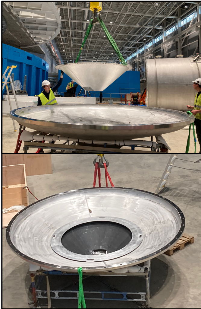
B 4 C lining in the tank nose cone
