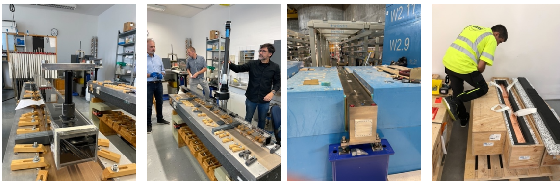
Figure 1. From left to right: 1-2, FAT of the second batch of out-of-bunker guides at TUM; 3, BWF installed; 4, NBOA inspection.
