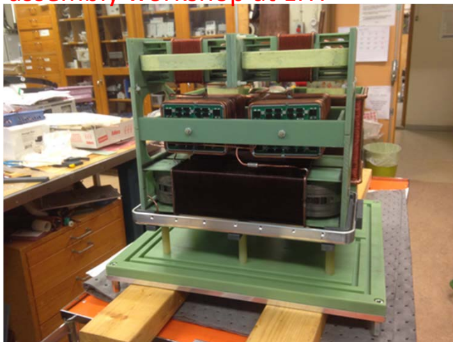
HV module prototype in assembly workshop at LTH
