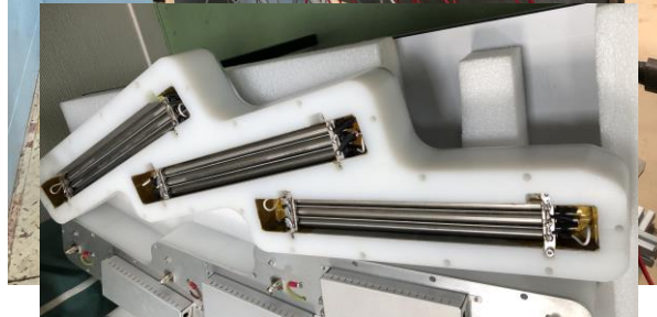
Triplets of triplets of 10 bar He-3 tubes
