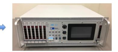
New tests were made with updated 3U/4U Verotech Caseframe chassis featuring airflow vents integrated into the top and bottom covers.
