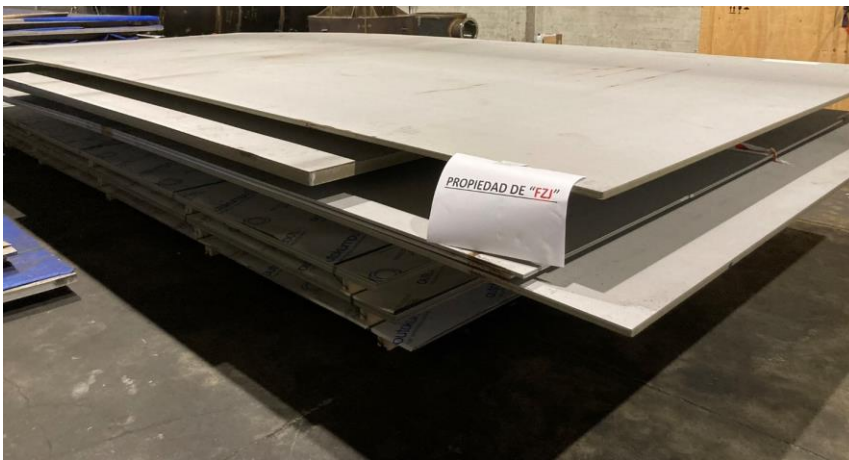
Figure 3: Raw material for the detector vessel at AVS
