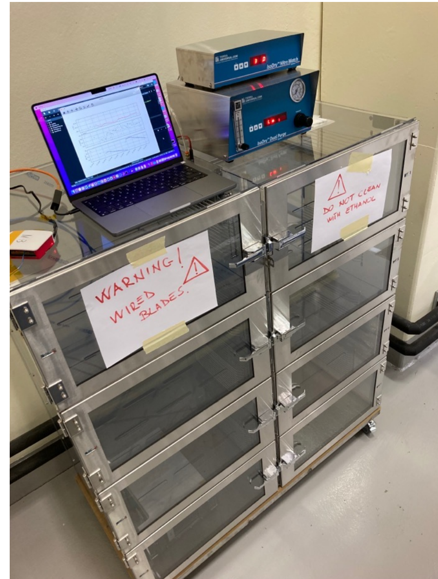
Blades kept in Nitrogen atmosphere Controlled via raspberry pi
