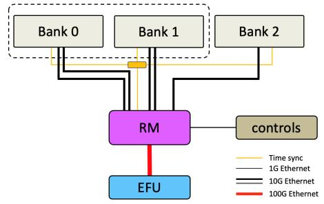
SKADI main system components and their data and control interfaces.
