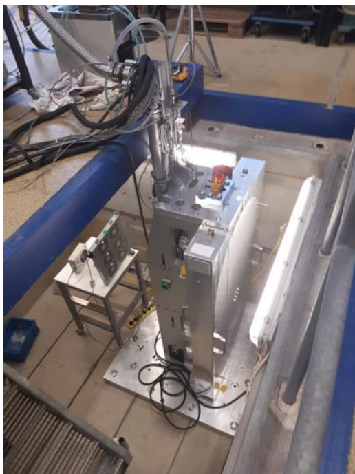
Figure 2: Fully assembled pulse-shaping chopper at the testing stand at FZJ
