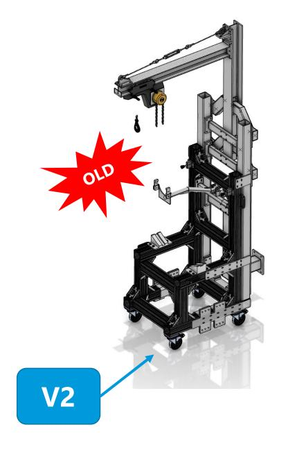
The crane will be mounted to both magnet supports acting as the main support of the crane avoiding flipping
