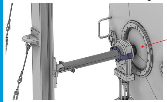
The mobile crane will be attached to the gate valve in order to avoid any movement.
