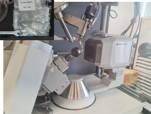
XRD One20DAC for preliminary HP studies ready for measurements using Single Crystal 4-circle diffractometer
