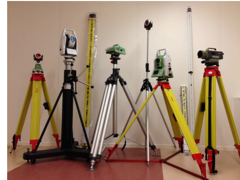
Instrumentation: laser tracker, total station, digital and optical levels, 3D Arm, GPS, metrology software.
