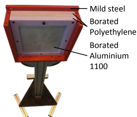
Figure 11. Photograph of an NDIFF instrument beam stop
