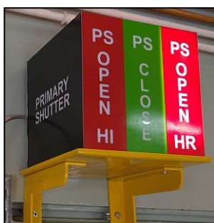
Figure 7. Photograph of the primary shutter status indicator.
