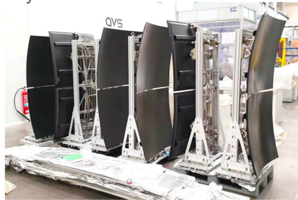
Panels and alignment for analyser system Si crystals tested at IN16B
