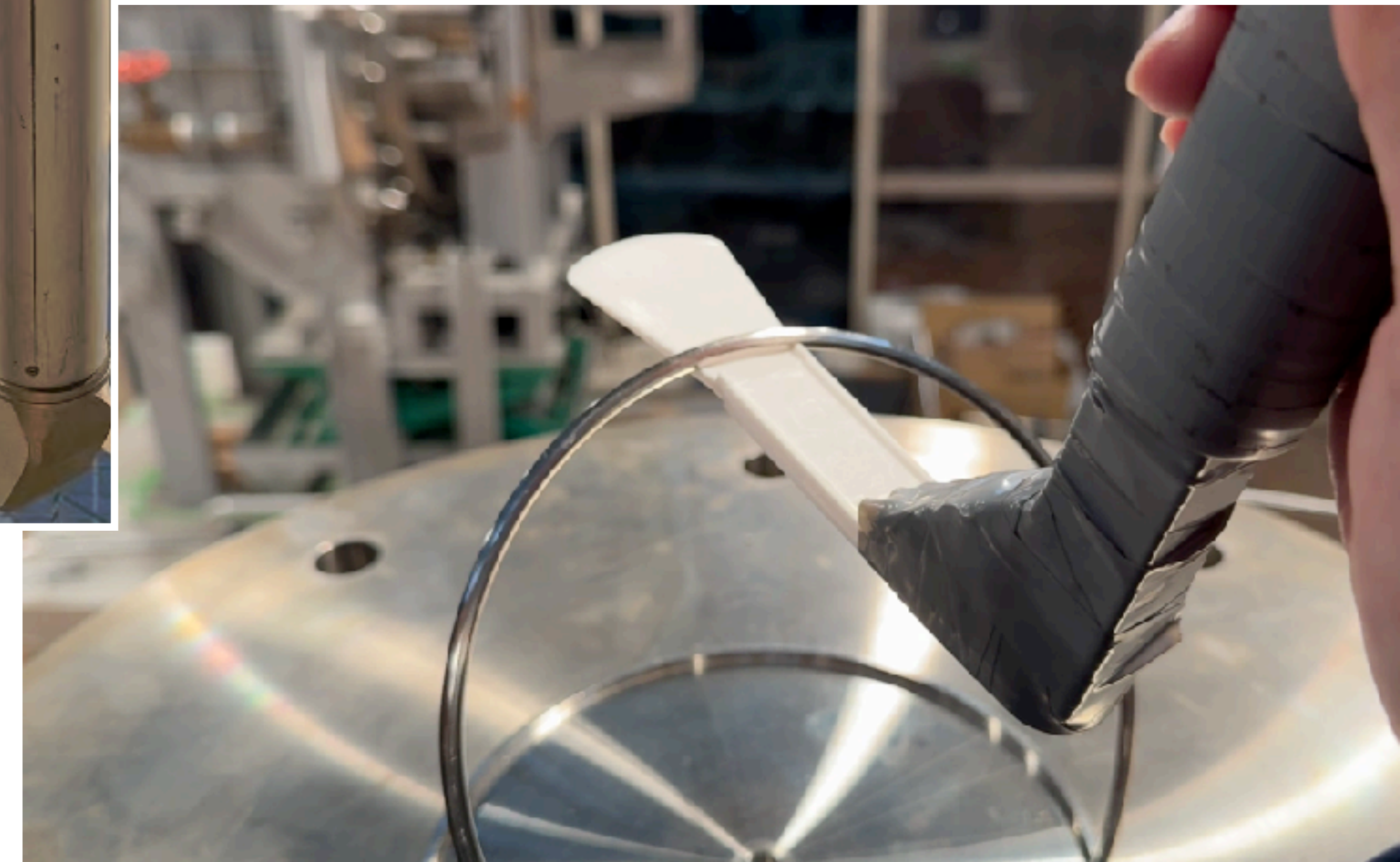
Metal seal replacement
