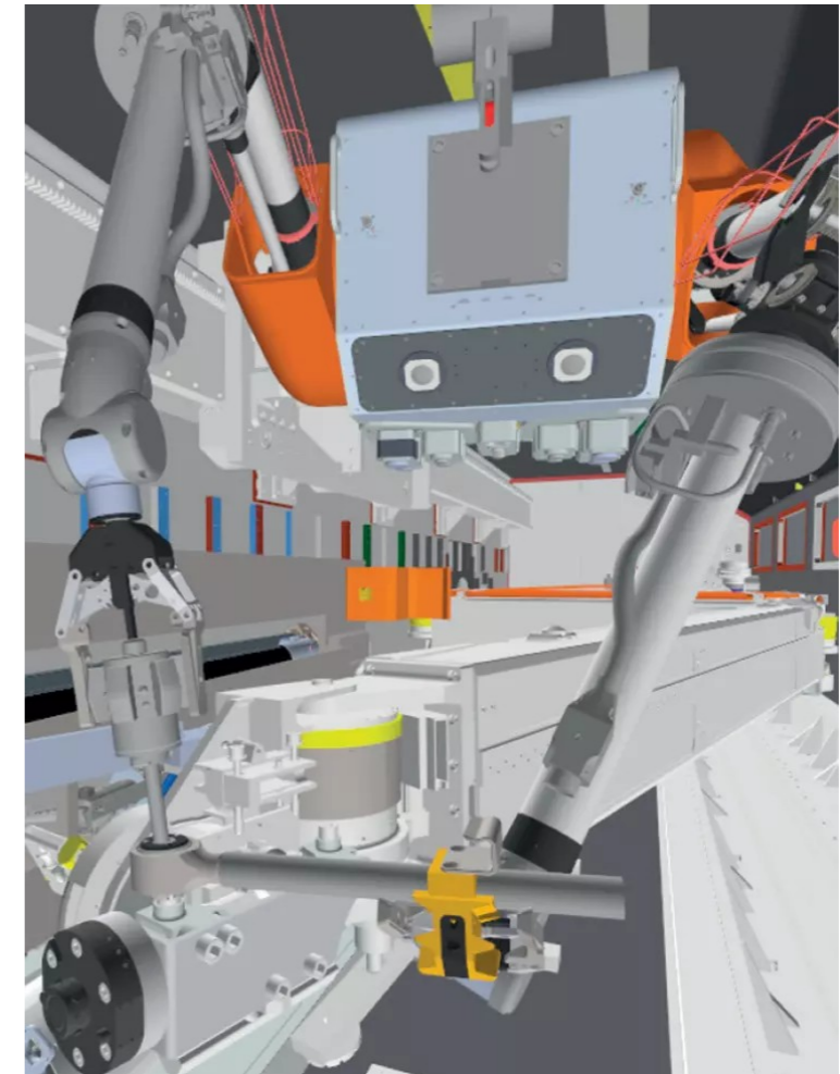
Figure 75: (left) Dexter Remote manipulator (Veolia Nuclear Solutions); (middle) one of the arms screwing a bolt; (right) Simulation of a robot operating at Fukushima.
