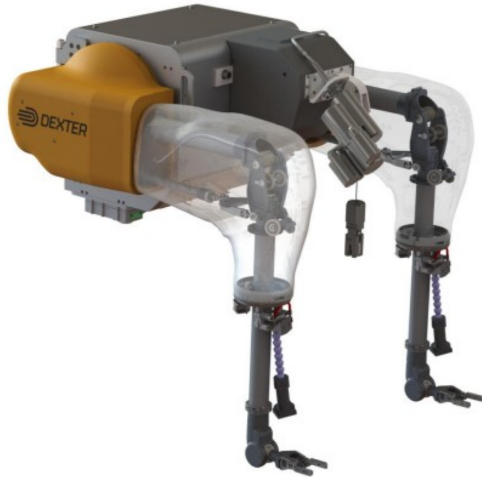
Figure 75: (left) Dexter Remote manipulator (Veolia Nuclear Solutions); (middle) one of the arms screwing a bolt; (right) Simulation of a robot operating at Fukushima.
