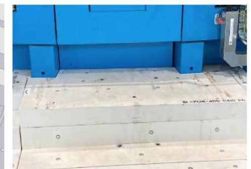
Photo 2 Interface LoKI shielding against bunker wall
