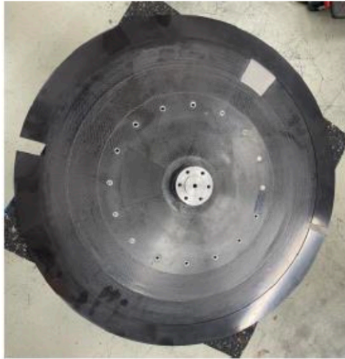
Figure 3: Left - M chopper disc M02 before test. Right - Test stand with remains from chopper disc after crash
