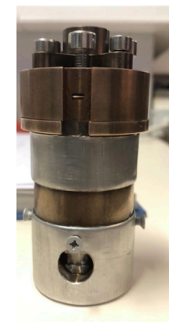
Figure 1. Photo of the 4 strain gauges and the PT100 thermometer which have been glued onto the CuBe cage. Photo taken before wires have been soldered.
