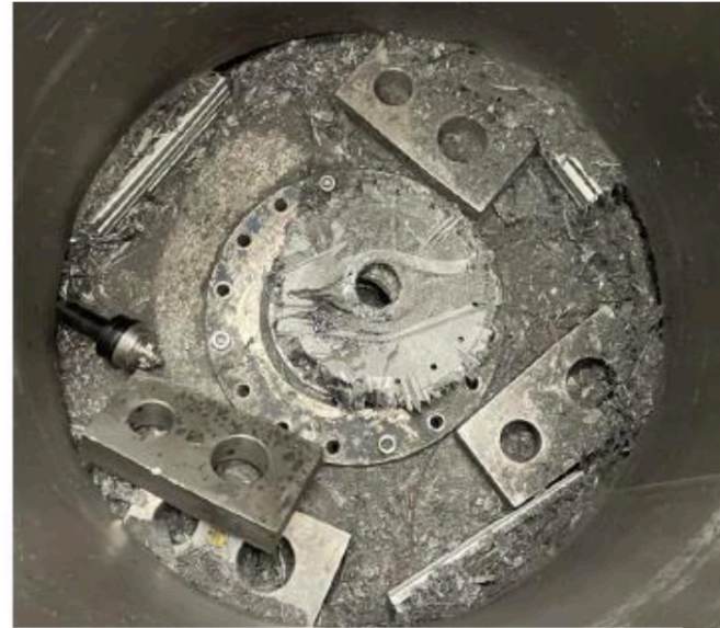
Figure 3: Left - M chopper disc M02 before test. Right - Test stand with remains from chopper disc after crash
