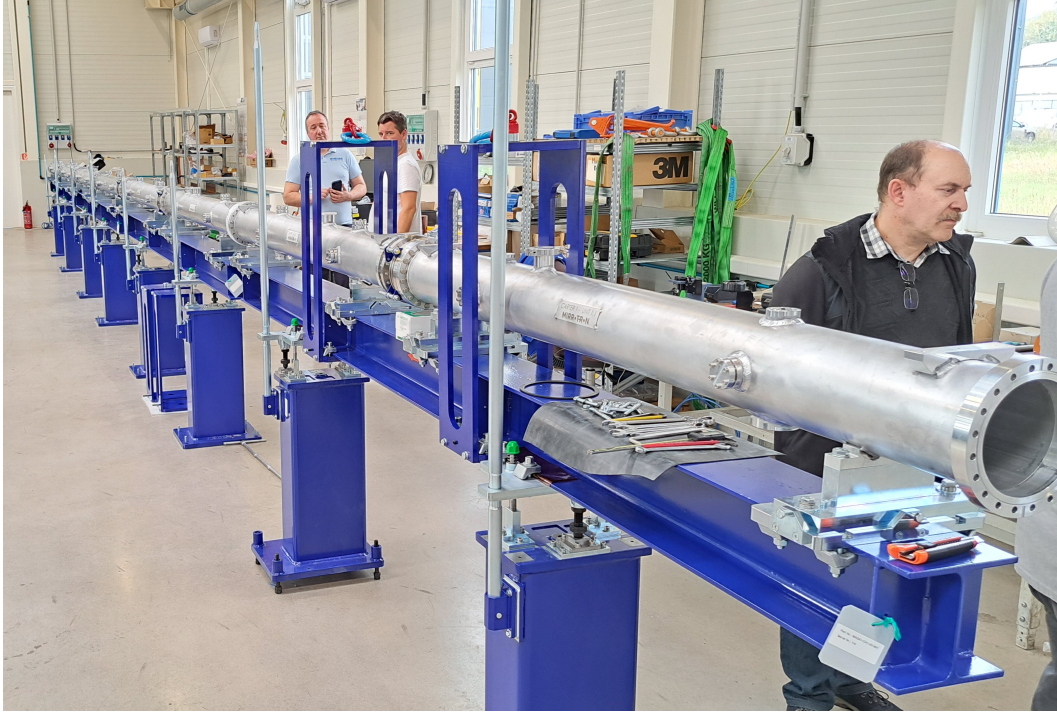
FIG. 2. The assembled in-Bunker Vacuum Housing at the Mirrotron facility.
