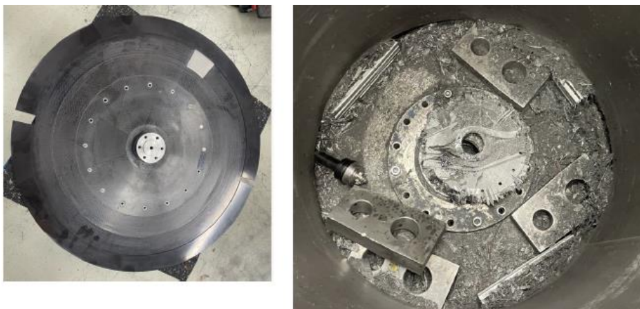
Figure 3: Left - M chopper disc M02 before test. Right - Test stand with remains from chopper disc after crash
