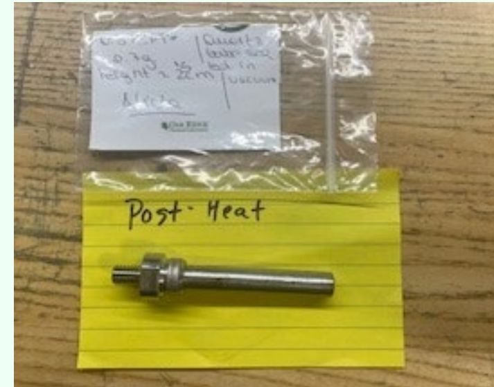
Test 2: Sample sealed in quartz capsule, inside of sealed vanadium sample can, heated to 750C for 2 hours
