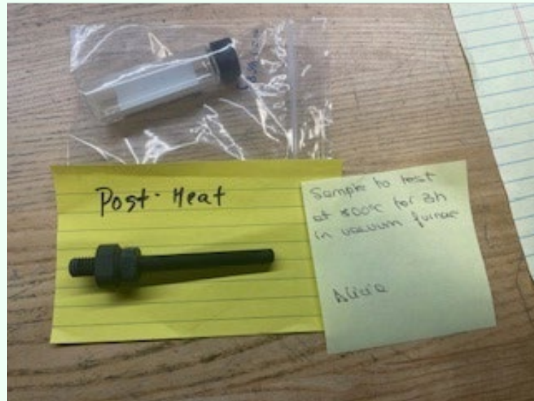
Test 1: Sealed Vanadium sample can heated to 800C for 3 hours
