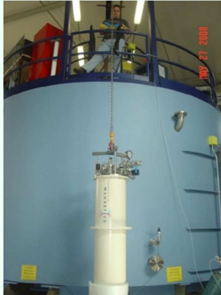
Installing 5 Tesla magnet onto BASIS (backscattering spectrometer) May 2008
