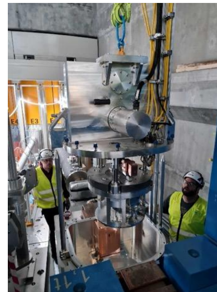
Chopper System (B4C Resin Al-disc, Diameter 700mm, 14Hz)
