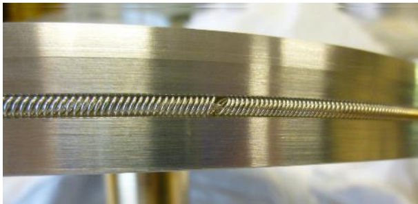
Mockup of the RF trap used for optimizing the grooves of the RF contacts
