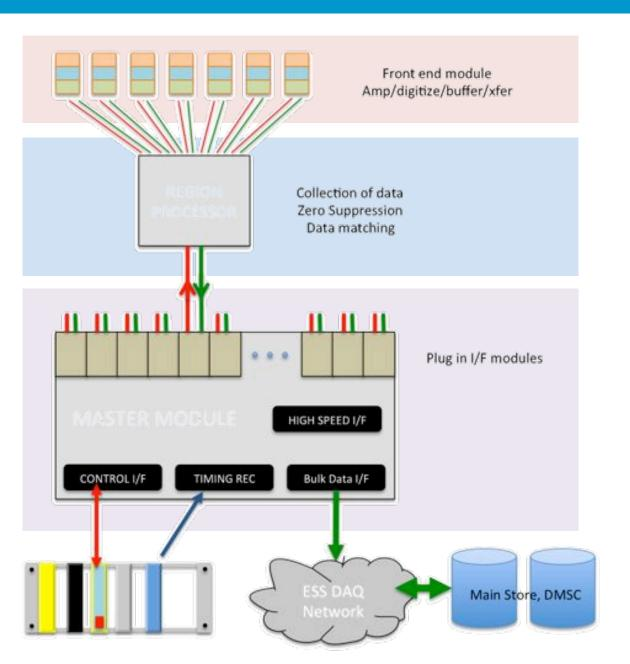
There are three logical layers in the generic readout layout. Not all layers are required in all instruments.
