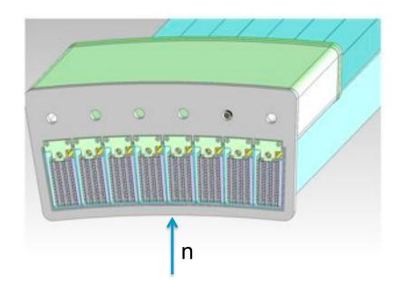
Electronics usually located at one end. Putting grid readout behind the column is also possible.
