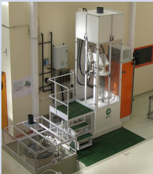
New Saclay vertical EP station: commissioned with 1.3 GHz single cell
