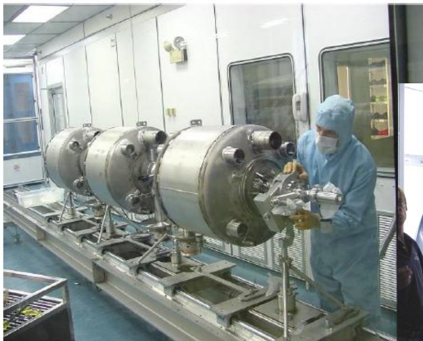
Figure 1: Typical assembly of a MB string.
