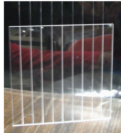
Proposal for the upgrade of CMS Hadronic EndCap Calorimeter (quartz plate and UV fibers)
