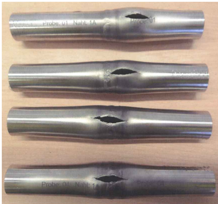
Burst test Invar-Invar welding
