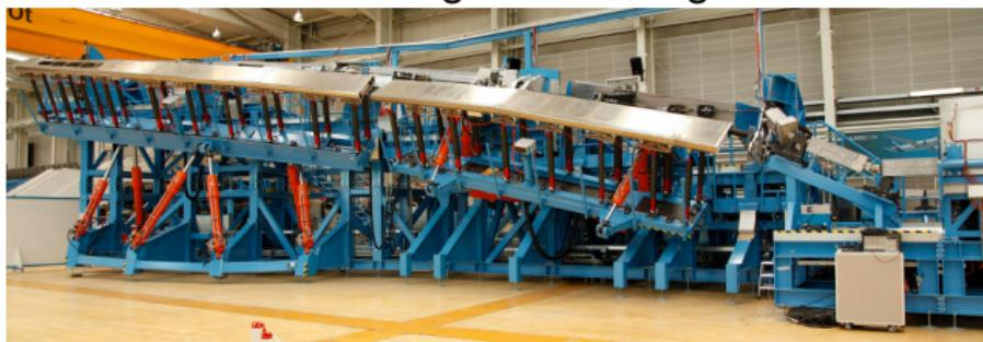
Airbus High-Lift Testrigs
