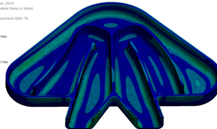
Equivalent stress (von Mises) @ 17 bar design pressure and 293 K
