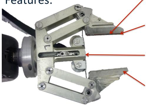
**Securing hole:** Accommodates a pin feature on gripped item so the item cannot be knocked out of grip
