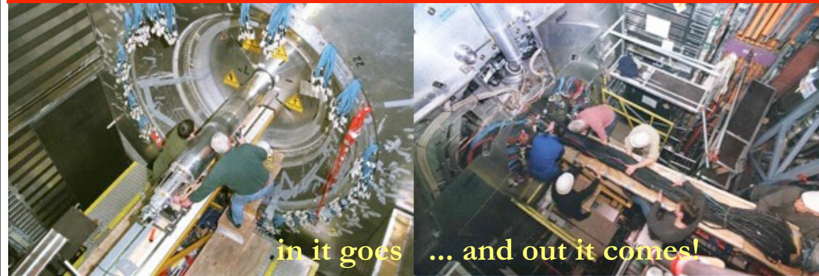
Installation of silicon microvertex detector
