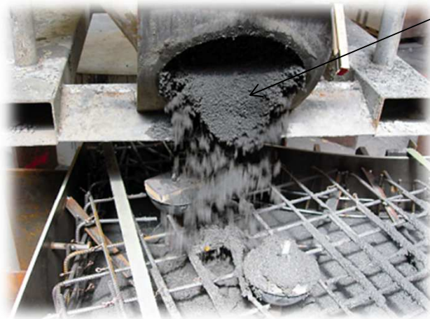
steel grains during pouring
