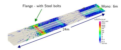
**Guide 1 day:** Activation from: Aluminium guide / Vacuum housing / Silicon windows
