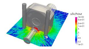
**T0-Chopper 7 day:** Activation from: Tungsten hammer / Inconnel rotor (80A) / Steel body
