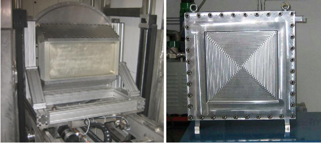
Figure 2: The Figaro detector [9] installed on the instrument (left) and a Denex detector [10] of active area of  $300 \times 300 \text{ mm}^2$  (right).
