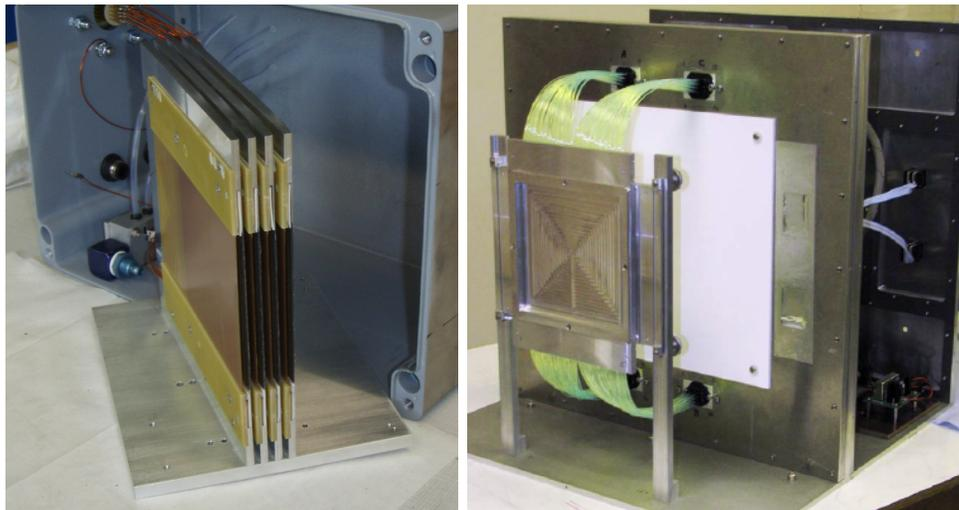
Figure 3: The Multi-Blade prototype developed at ILL (left). The WLS scintillating detector developed at ISIS (right).
