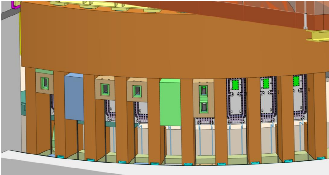
Figure 14 Version of the assembly with orange, permanent, shielding between and above ports. There is a 390mmx494mm wide handling area at all ports. The bit above the ports extends out of the R6000mm
