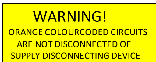
Figure 1 - Circuits not disconnected of supply disconnecting device
