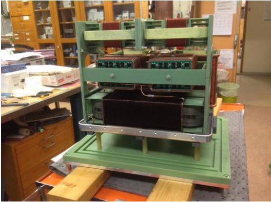
Figure 7: Open view of high voltage module
