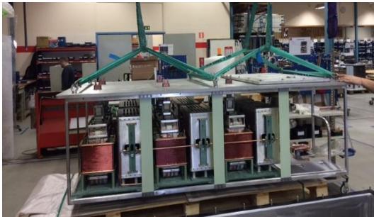
Figure 8: Open view of high voltage oil tank assembly
