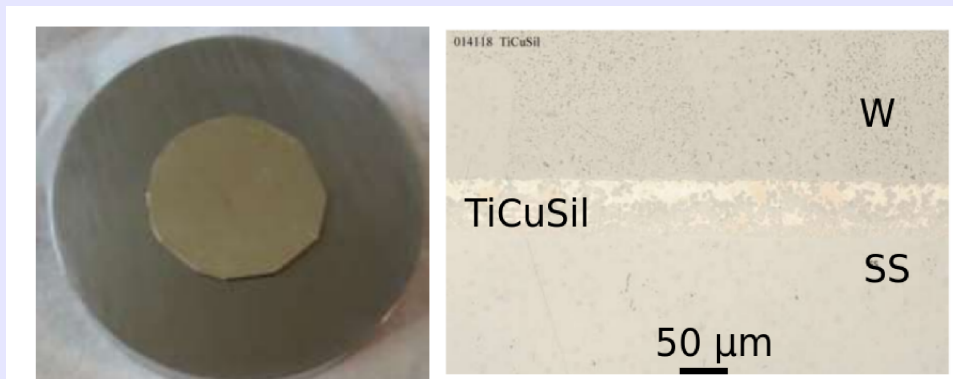
Figure 12. Brazing of Tungsten blocks- current status. Compare [2].
