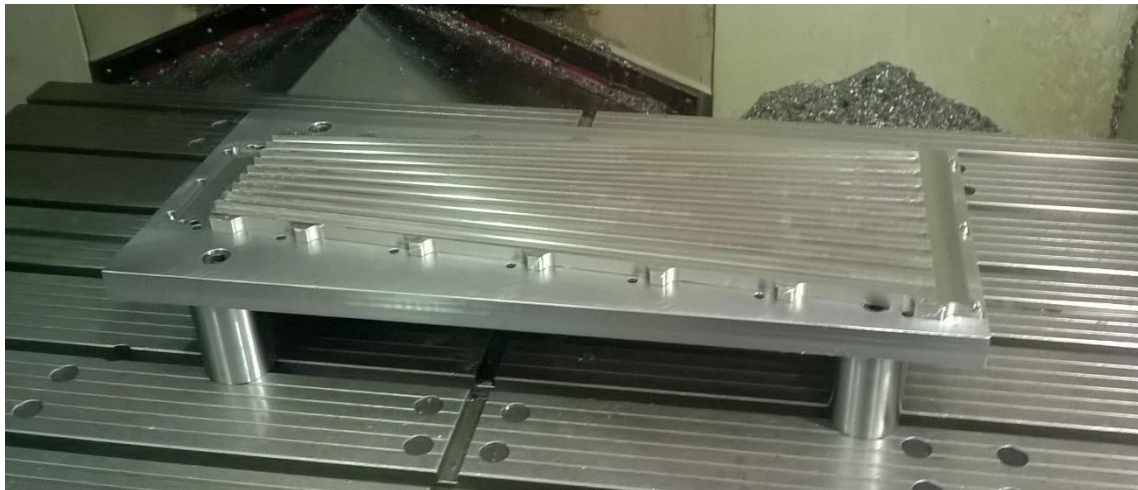
Tooling for upper and lower plate machining
