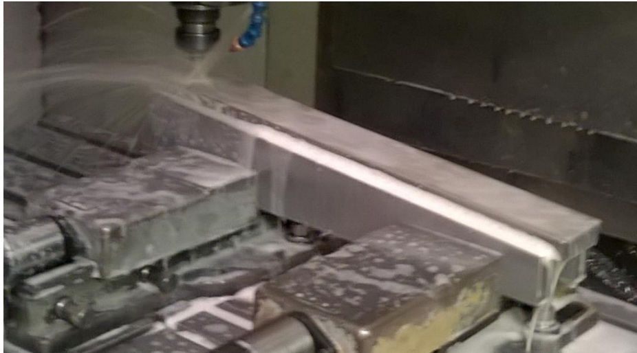
Side wall inside milling machine
