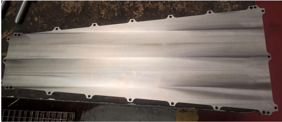
Special clamping in upper plate to avoid bending
