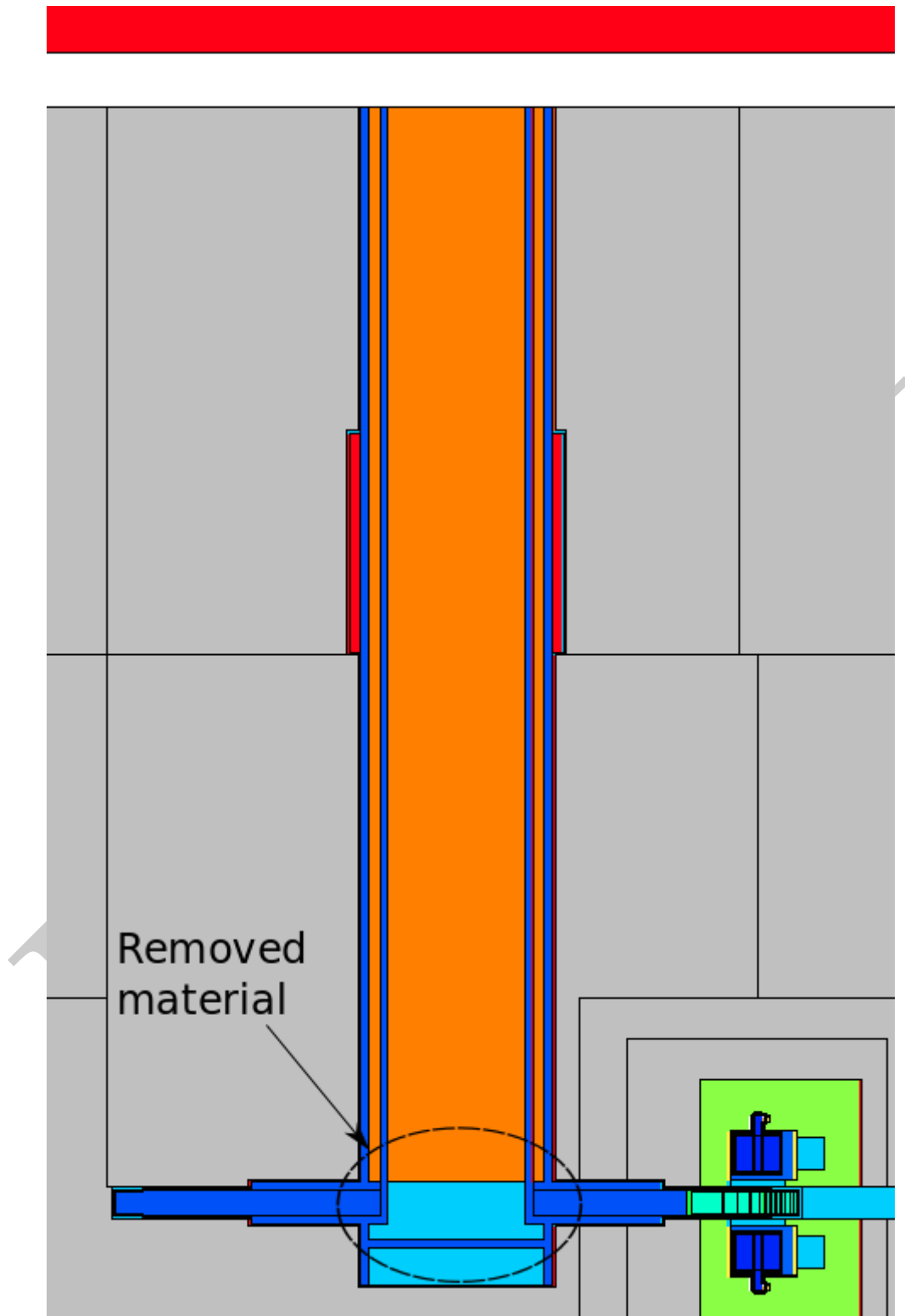
Figure 3.15: Configuration of removing the bottom part of the shaft shielding.
