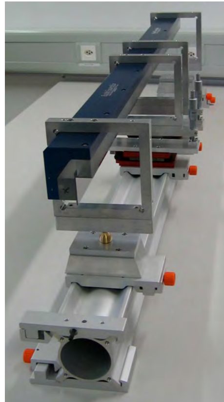
Figure 11.6: Guide support with 2 guide elements mounted. Shown is the second guide of the Selene set-up, reflecting left and downwards. The guides are not yet adjusted, the knife blade slit is missing.
