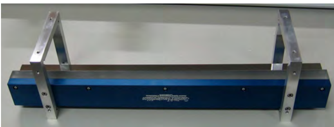
Figure 11.7: Single guide element (half a guide section). The blue part is an L-shaped Al bar on which the glass substrates are screwed. The Al frames are for mounting the elements on the support and alignment system.
