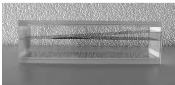
Figure 7.2: Left: First sketch for a frame-overlap filter and polariser for the Selene prototype set-up, based on transmission/reflection through/at spiral-curved surfaces. Right: Final device, produced by SwissNeutronics. The glass tube is 215 mm long and has an inner height and width of 50 \times 50 \text{ mm}^2 . The virtual source is to be 170 mm before the entrance (to the left).
