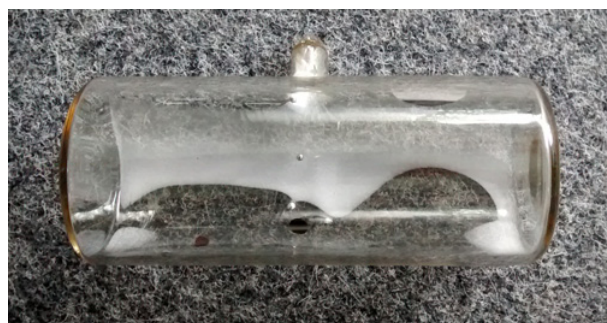
Figure 3. An example of a ^3\text{He} spin filter cell prepared for TOPAS.
