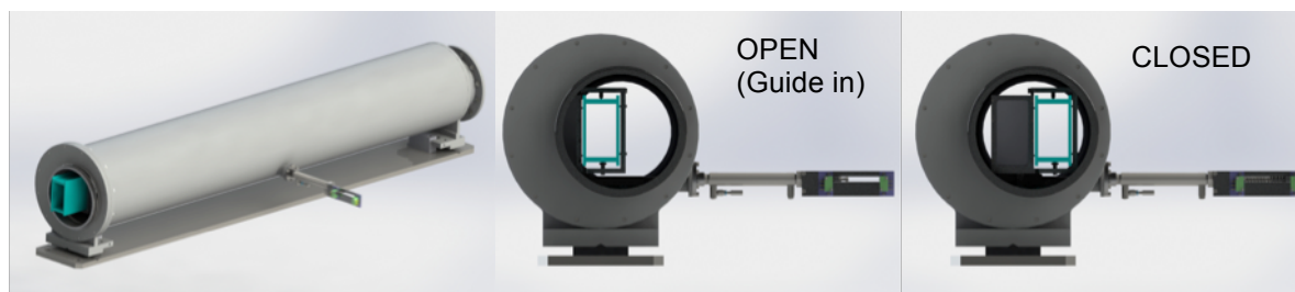
Figure 5. Proposed Heavy Shutter Concept.
