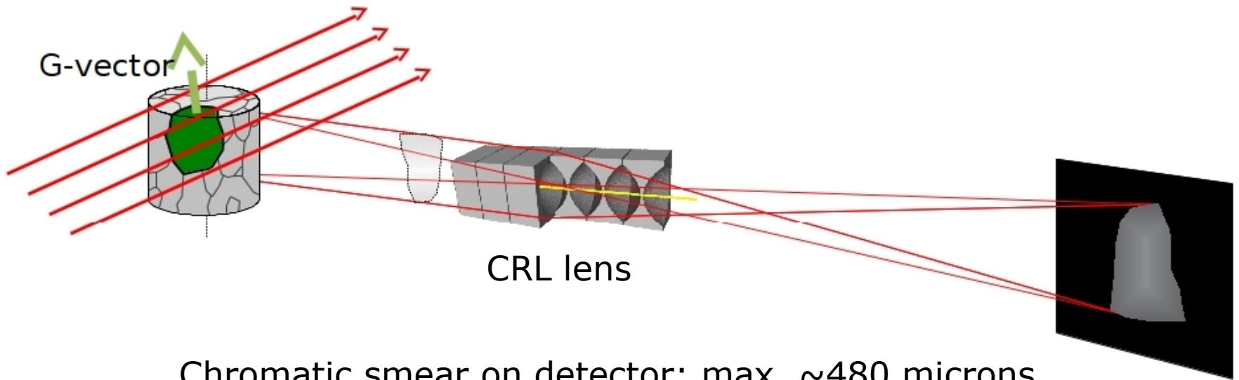
Chromatic smear on detector: max.  $\sim 480$  microns
