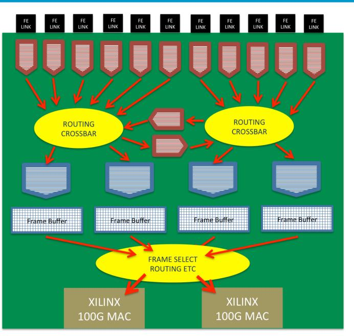
Data from front end links (24 max speed 10G/25G)
