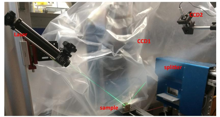
**Geometric reconstruction** of sample surface position and angle
