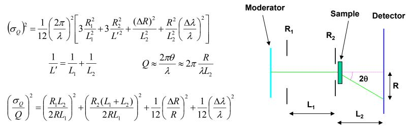
"Optimal" SANS - best flux for best Q resolution:  $L_1 = L_2$ ,  $R_1 = 2R_2$
