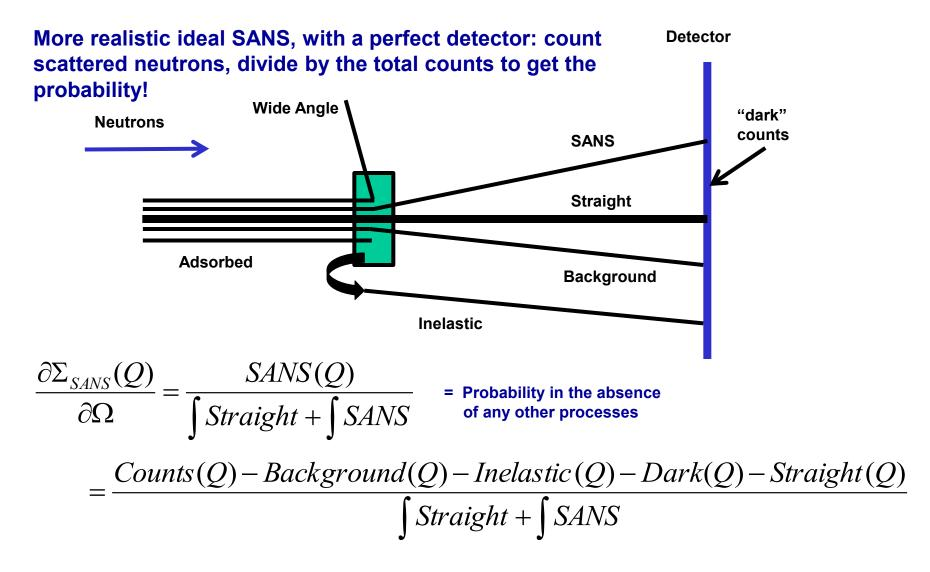
No transmission measurement or detector efficiency is needed (until we get to larger scattering angles!)
