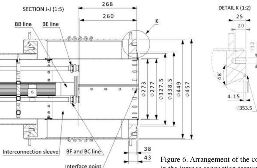
Figure 6. Arrangement of the cold process pipes in the jumper connection termination - side view
